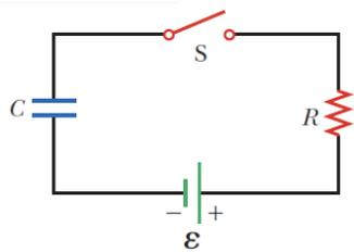
35. A  $2.00\text{-nF}$  capacitor with an initial charge of  $5.10 \mu\text{C}$  is discharged through a  $1.30\text{-k}\Omega$  resistor. (a) Calculate the current in the resistor  $9.00 \mu\text{s}$  after the resistor is connected across the terminals of the capacitor. (b) What charge remains on the capacitor after  $8.00 \mu\text{s}$ ? (c) What is the maximum current in the resistor?
