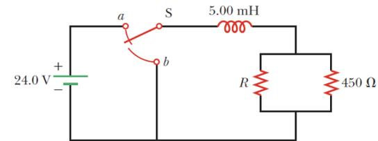
21. The switch in Figure P32.21 is open for  $t < 0$  and is then thrown closed at time  $t = 0$ . Assume  $R = 4.00 \Omega$ ,  $L = 1.00$  H, and  $\mathcal{E} = 10.0$  V. Find (a) the current in the inductor and (b) the current in the switch as functions of time thereafter.
