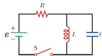
44. Calculate the inductance of an  $LC$  circuit that oscillates at  $120\text{ Hz}$  when the capacitance is  $8.00\ \mu\text{F}$ .
